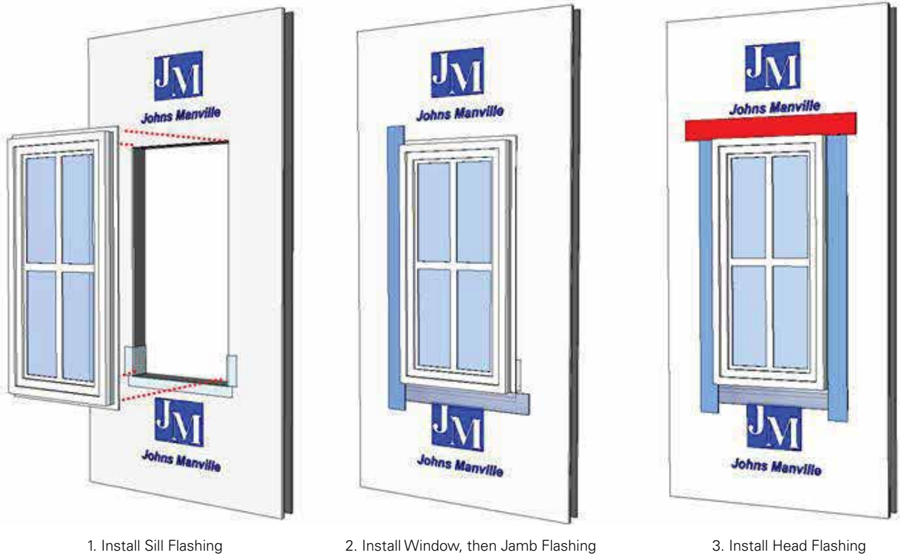
FIGURE 4. TYPICAL PENETRATION FLASHING DETAIL - FLANGED
